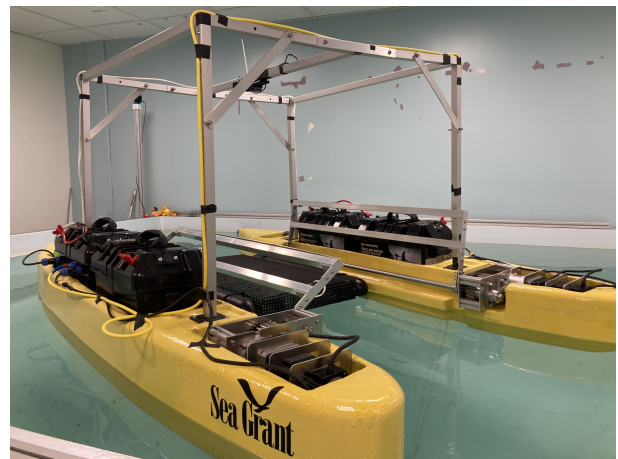
Fig. 1. The 2023 Oystermaran in the lab. Note the oyster basket between the hulls and the two flipping arms.
